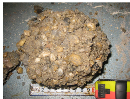
图 4 灌浆后结石体 Fig.4 Calculus after grouting
